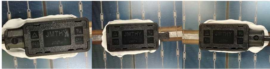
Fig. 3: View of junction box of module type ERA Pro-72HCB575M
